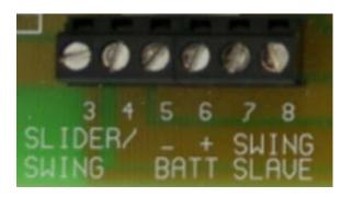
The Master motor (motor 1) is connected to terminals 3 & 4 (SLIDER SWING), and the slave motor (motor 2) is connected to terminals 7 & 8 (SWING SLAVE).
