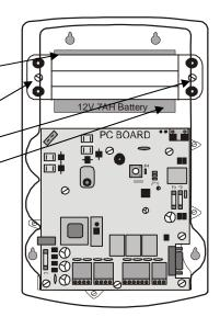
STEP 4: Drill 4 x 8mm holes for mounting the unit. Four nail-in anchors are supplied with the unit. Insert the plastic sleeve of the nail-in anchor from the inside of the box and then hammer the screw in with a screw driver and hammer.
