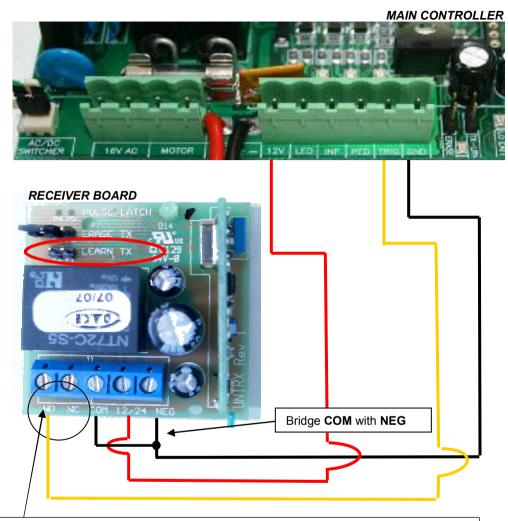
Connect N/O to the TRIG input for full opening or the PED input for pedestrian opening
