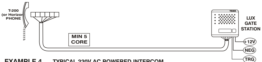
EXAMPLE 4 TYPICAL 220V AC POWERED INTERCOM
